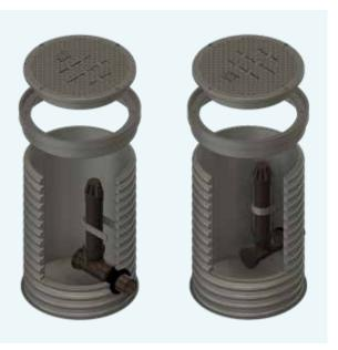
Fitted with a 110mm overflow pipe complete with debris cowl, the pipe and cowl can be removed if the orifice becomes blocked which allows the system to drain down and the blockage removed.
